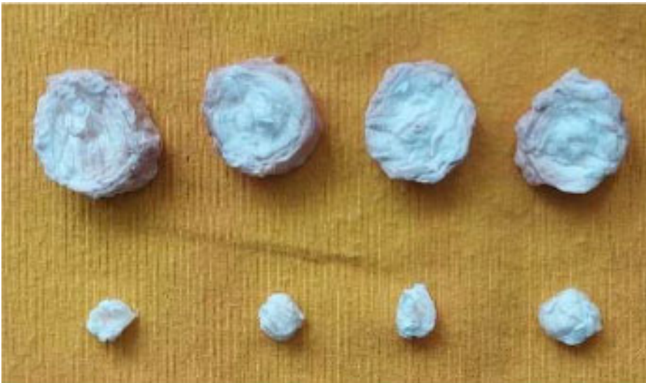
Figure 3. The final result of freeze-drying is that the material is dry and resembles a freeze-dried cake.
